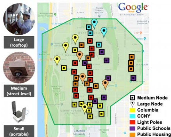
Figure 3. COSMOS Base Station Deployment Plan
